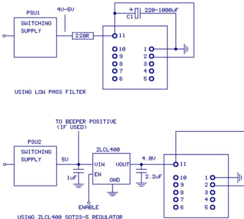
The upper diagram shows a low pass filter which may help increase range if the output ripple from the switching power supply is less than 10mV PKPK. The best solution, and the one which takes up
